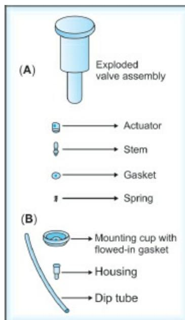
**Figs 21.1A and B:** (A) Vapour tap body; (B) Aerosol can valve assembly
