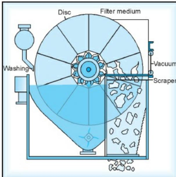
**Fig. 5.5:** Disc filter
