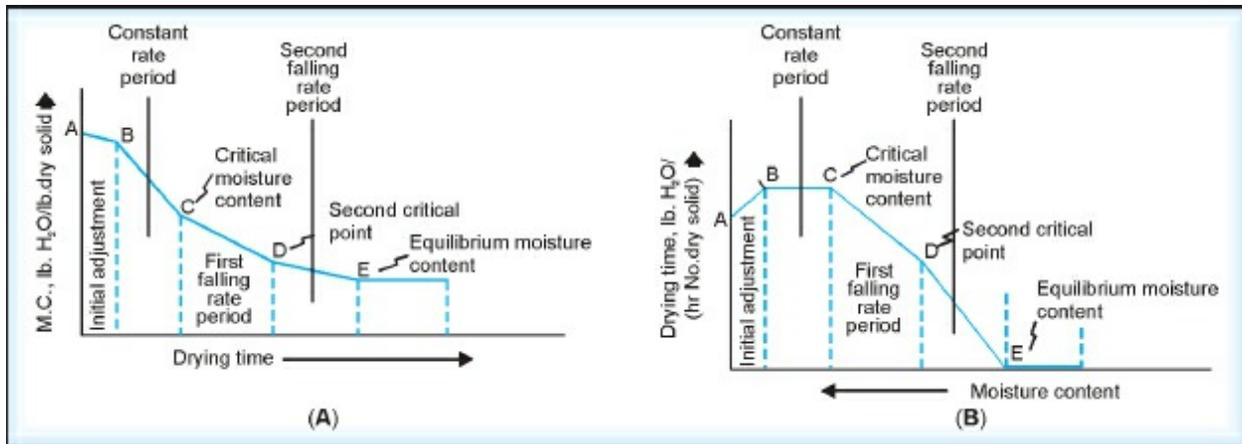
**Figs 4.1A and B:** The stages of drying
