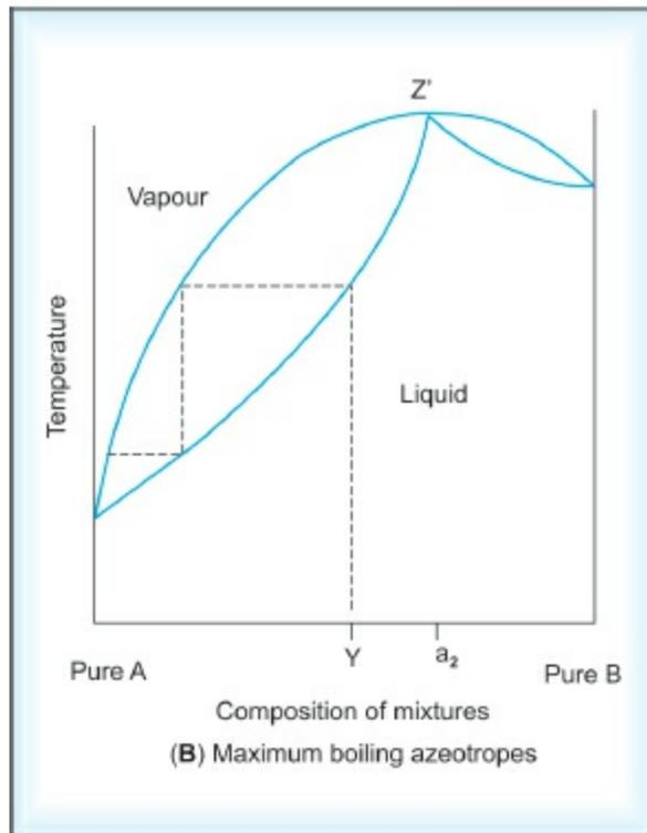
**Figs 3.13A and B:** Boiling point diagrams of minimum and maximum boiling azeotropes: (A) Minimum boiling azeotropes, (B) Maximum boiling azeotropes
