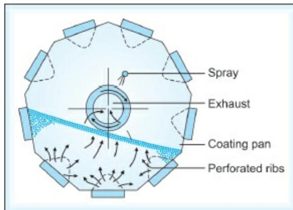
**Fig. 13.29:** Line diagram of driacoater pan
