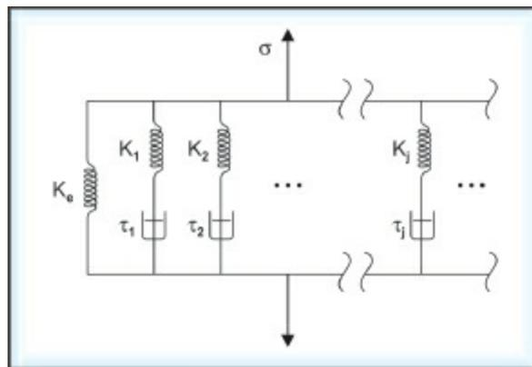
**Fig. 6.30:** Diagrammatic representation of the Weichert model
