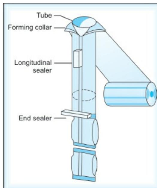
**Fig. 27.9:** Vertical form/fill/seal system
