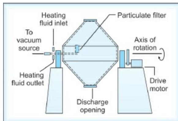
**Fig. 4.10:** Rotating double-cone vacuum dryer
