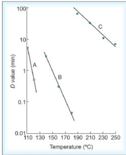
**Fig. 22.2:** Z-value plots of log  $D$  versus temperature
