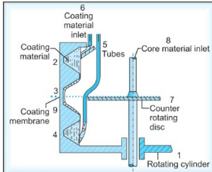
**Fig. 15.16:** Sectional diagram of multiorifice-centrifugal microencapsulation apparatus
