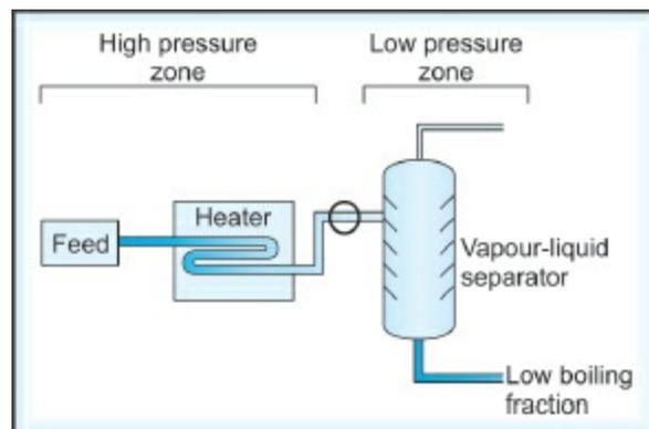
**Fig. 3.17:** Diagrammatic representation of a flash distillation unit
