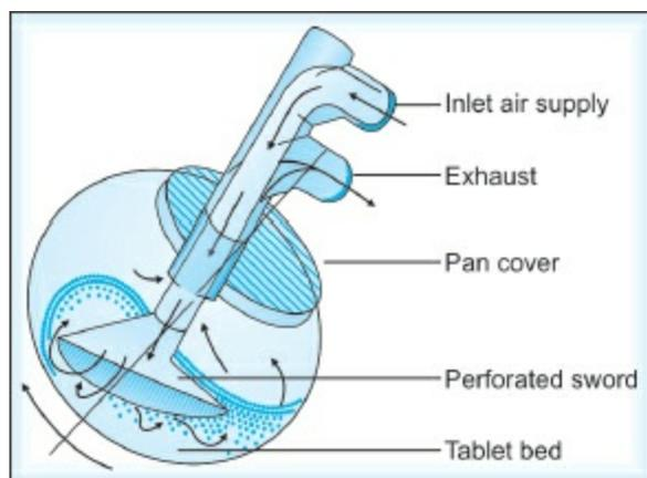
**Fig. 13.25:** Line diagram of Glatt immersion-sword system
