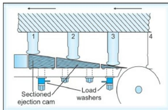
**Fig. 13.61:** Instrumented ejection cam. Diagram shows the preferred method of sectioning an ejection cam and the transducer locations for monitoring ejection forces on a multi-station tablet press
