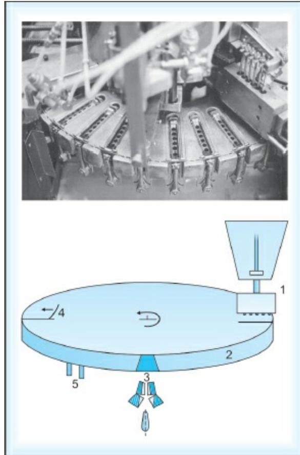
**Fig. 20.4:** Rotary suppository molding machine, (1) feeding device and filling hopper, (2) rotating cooling turntable, (3) suppository ejection station, (4) scraping device, (5) refrigerant inlet and outlet
