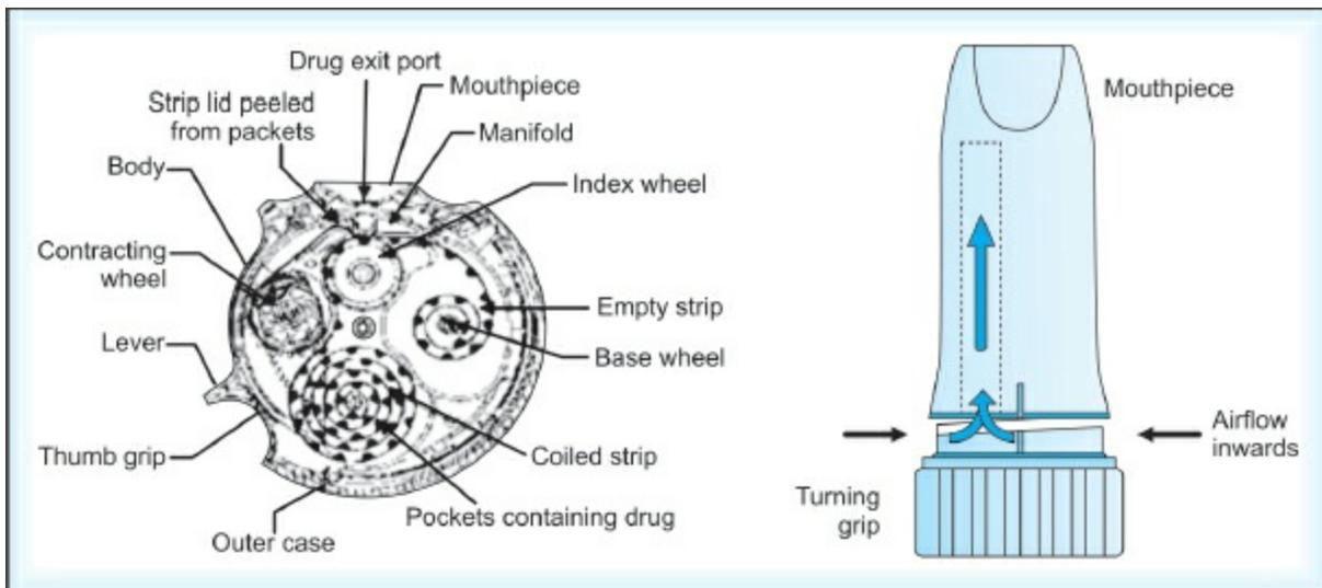
**Fig. 21.18:** A simplified view of the Diskus<sup>®</sup> and a Turbuhaler DPI
