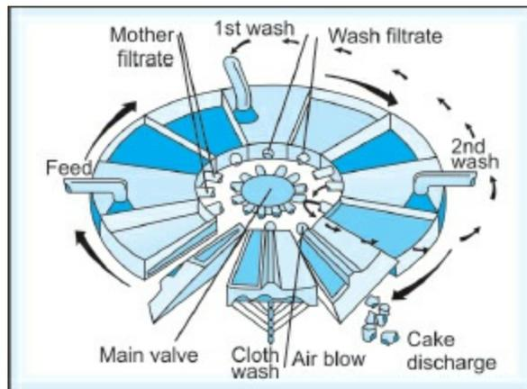
**Fig. 5.7:** Schematic representation of tilting pan filter
