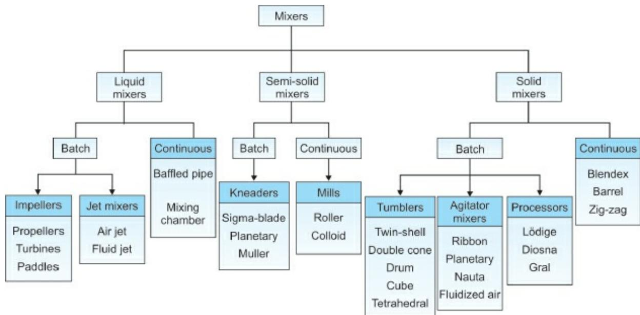
**Fig. 1.1:** Classification tree of mixing equipments
