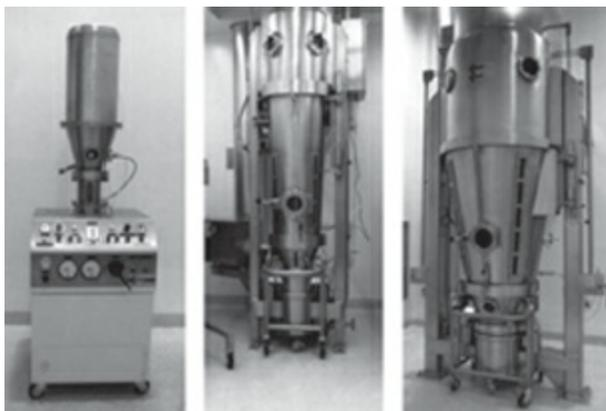
**Fig. 26.9:** Fluidized-bed dryers of 1,5 and 50 kg capacity
