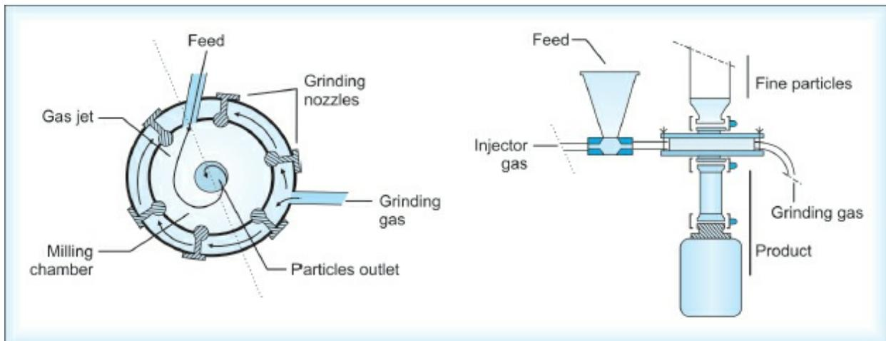
**Fig. 2.15:** Diagrammatic representation of spiral jet mill
