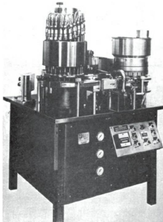
**Fig. 14.13:** Perry model CF ACCOF1L capsule filling machine (*Courtesy of*
