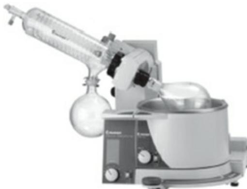
**Fig. 3.10:** Laboratory scale rotary evaporator
