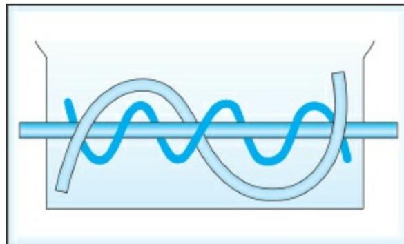
**Fig. 1.19:** Side view of a top-loading ribbon blender
