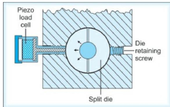
**Fig. 13.56:** Piezo-electric die wall instrumentation. An example of the use of a piezo-electric force transducer (in a special holder) in conjunction with a vertically split die to measure radial die wall forces
