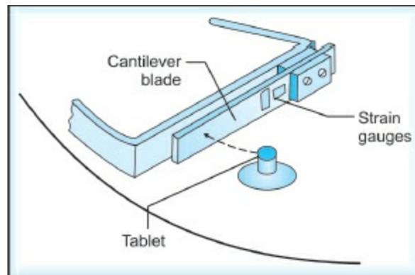
**Fig. 13.62:** Instrumentation to measure “sweep-off” force. Diagram illustrates measurement of the force of adhesion between a tablet and the lower punch of a tablet press by means of a strain-gauged cantilever blade attached to the feed frame
