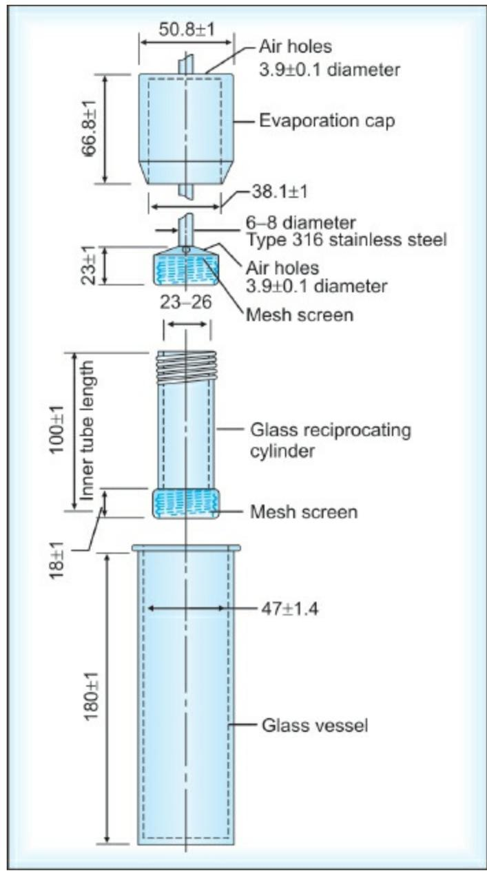
**Fig. 8.8:** USP apparatus 3 (reciprocating cylinder apparatus)
