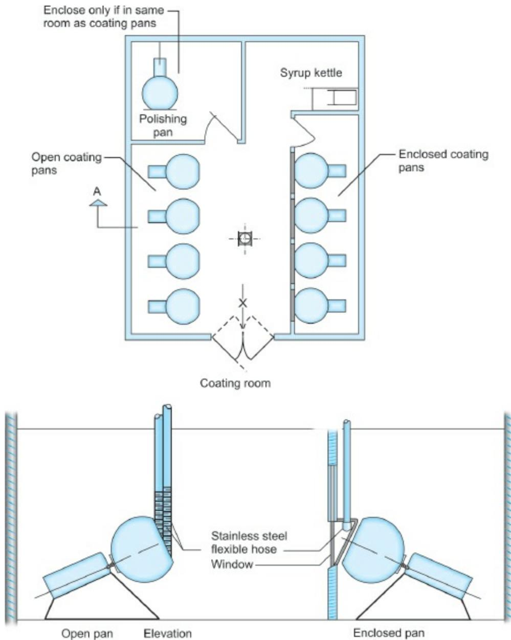
**Fig. 26.17:** Top, An enclosed bank of coating pans. Polishing pans should be in a different location from coating pans. Bottom, Differences between open and enclosed pans.
