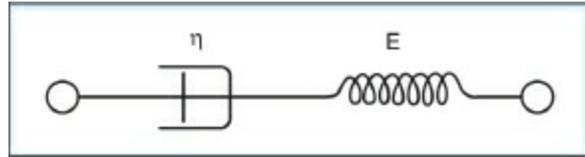
**Fig. 6.27:** Diagrammatic representation of the Maxwell model
