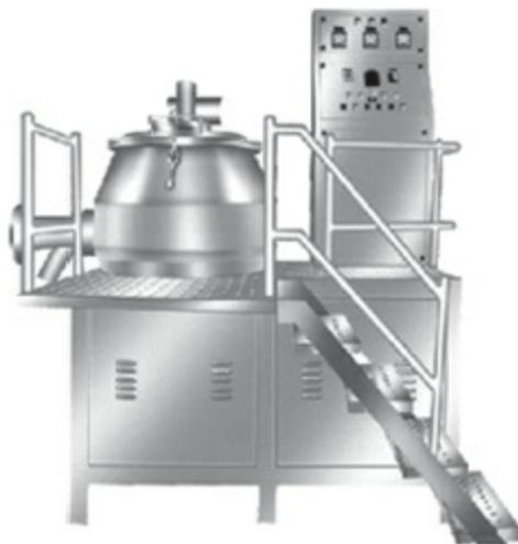
**Fig. 26.8:** High-shear pharmaceutical grade mixer/granulator
