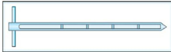
**Fig. 1.26:** Diagrammatic representation of a sampling thief
