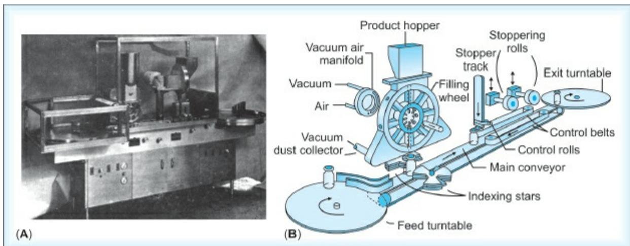
**Figs 23.11A and B:** (A) Automated filling unit for dry solids. The operation is protected by hoods to maintain an aseptic environment; (B) The diagram represents the functioning parts with the unscrambler turntable at left, the filling machine, the rubber closure inserting device, and the collecting turntable for the filled and stoppered vials at right
