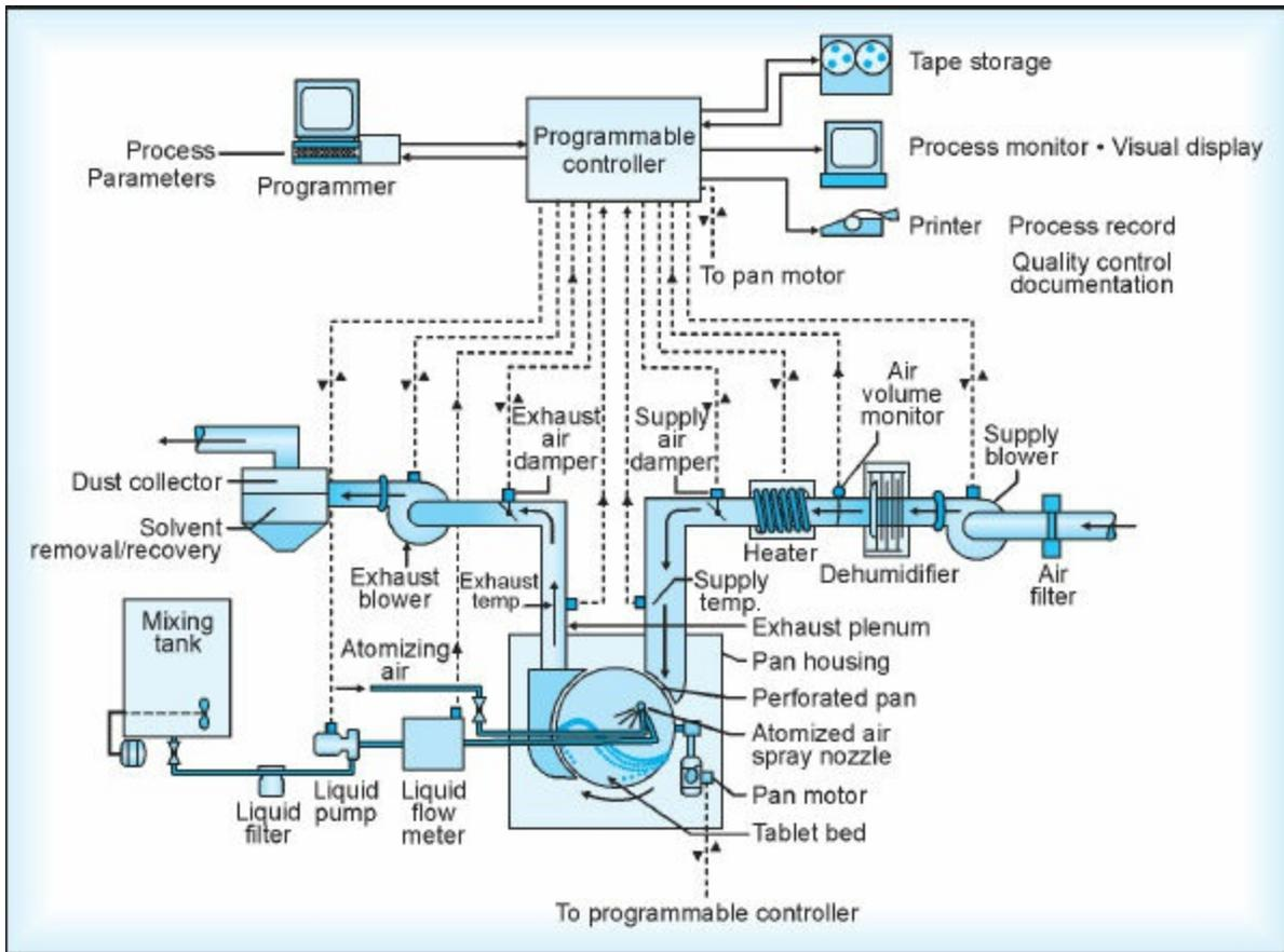
**Fig. 13.35:** Diagram of an automated coating system
