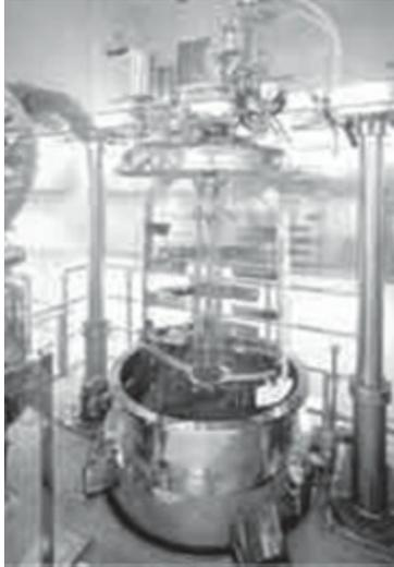
**Fig. 19.9:** The high shear homo-mixer is attached to an electrically driven lift mechanism for raising or lowering it into the jacketed kettle used for dispersing solids in liquids
