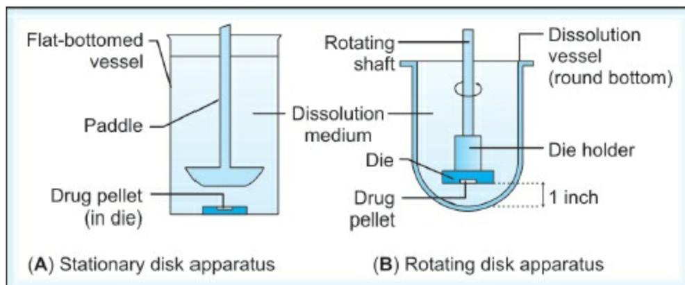
**Figs 8.5A and B:** Schematic representation of intrinsic dissolution apparatus: (A) Stationary disk apparatus; (B) Rotating disk apparatus
