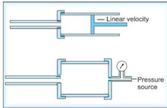
**Fig. 6.17:** The extrusion rheometer. Either a constant linear velocity is imparted to the piston to give a preset volume delivery and the piston force is measured, or a preset force (air pressure) is applied and the rate of volume delivery is determined
