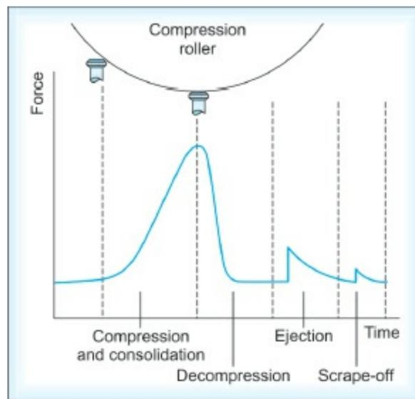
**Fig. 13.39:** The schematic representation of the compression process
