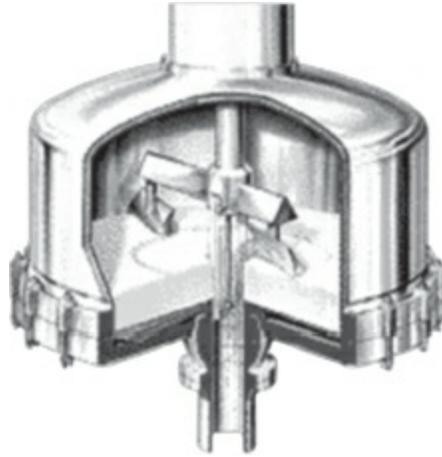
**Fig. 5.8:** Schematic representation of Nutsche filter
