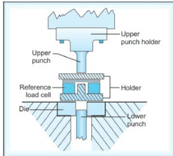
**Fig. 13.57:** Calibration using load cell. Diagram illustrates the use of a piezoelectric transducer and special holder to calibrate the upper and lower punch instrumentation on a single-station press
