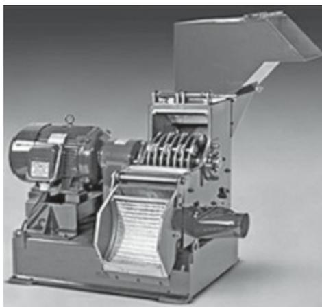
**Fig. 26.11:** Hammer mill (comminuting machine). The comminuting action occurs inside the mill head, where the high-speed centrifugal force of the blades hurls the granulation through the screen, which is held in place at the
