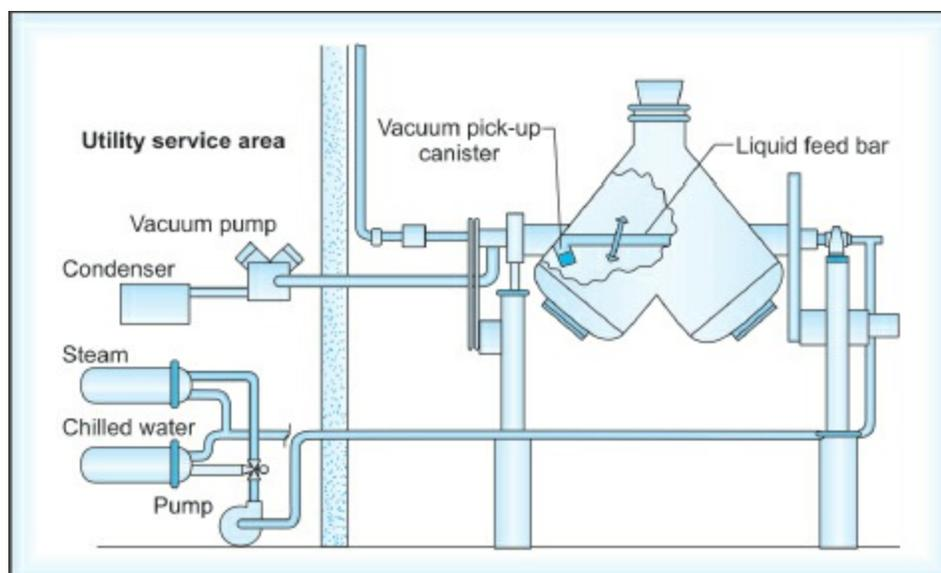
**Fig. 26.14:** Schematic of a multifunction pharmaceutical processor. The system contains a solids mixing shell, which includes a liquid dispersion bar. This unit is jacketed to allow heating and cooling. Material can be dried within the unit by use of the vacuum canister and condenser
