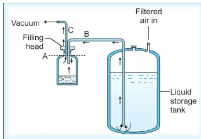
**Fig. 17.11:** Schematic diagram of the principle used in vacuum filling. The vacuum drawn through tube C reduced pressure in the container. Pressure differential causes liquid in storage tank to flow through tube B into container. When liquid level reaches point A, excess is carried out through tube C and may be recycled to liquid storage tank
