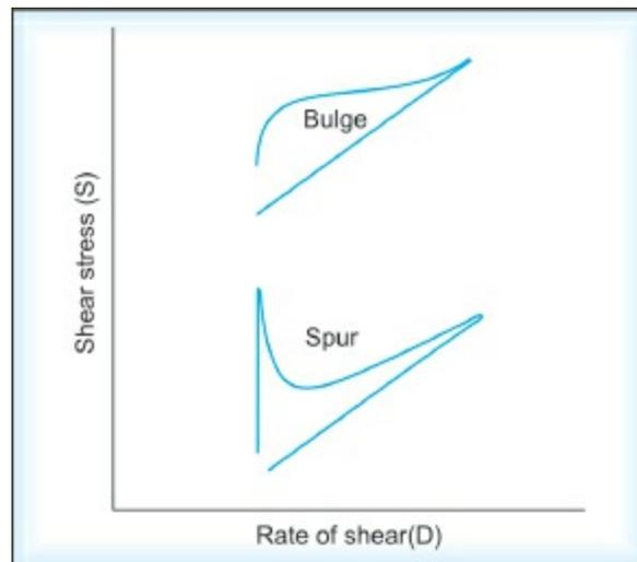
**Fig. 6.13:** Rheogram for a thixotropic material showing bulge and spur in the hysteresis loop
