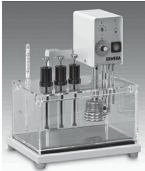
**Fig. 20.6:** Assembly for measuring the softening time of suppositories
