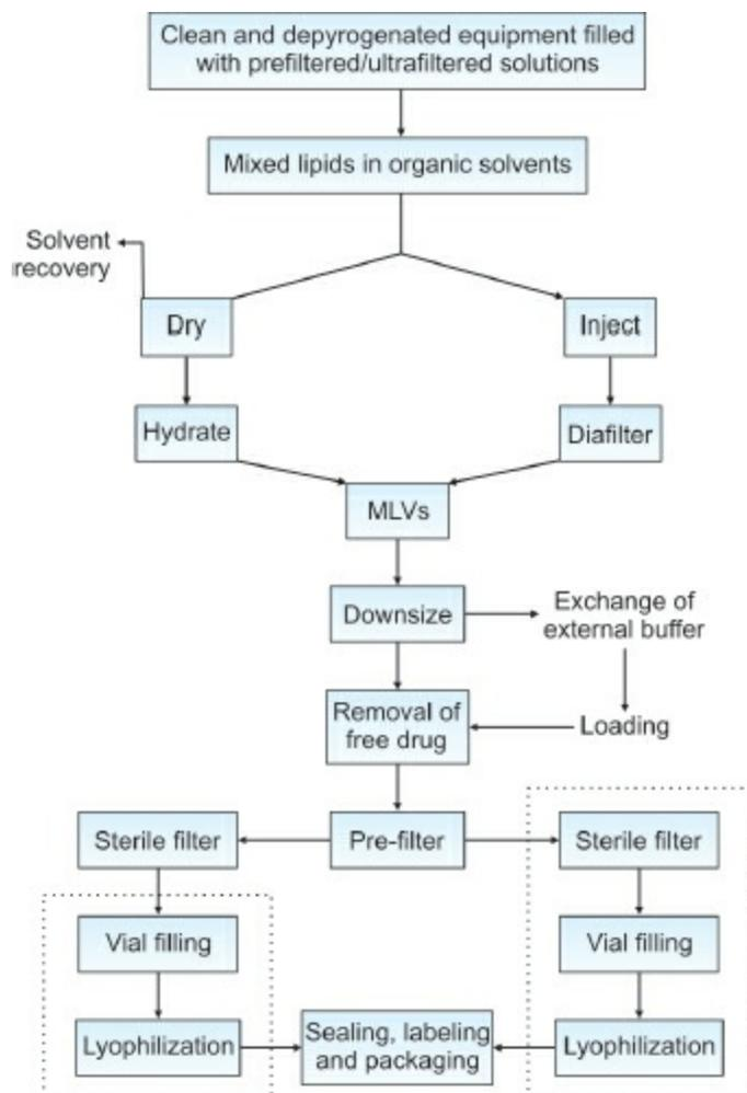
**Fig. 24.18:** Various steps for the commercial manufacturing of liposomes (Doxil™). Steps indicated in the box with discontinuous lines should be performed under the aseptic conditions
