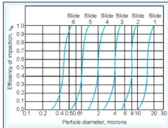
**Fig. 21.14:** Impact efficiency of cascade impactor (model CI-S-6)
