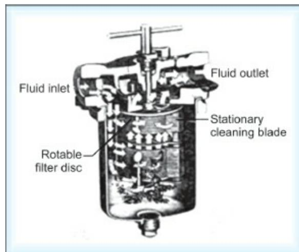
**Fig. 5.12:** An edge filter with automatic cleaning device may be automated by replacing handle with motor
