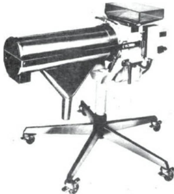
**Fig. 14.17:** Erweka KEA capsule dedusting and polishing machine (*Courtesy of Erweka-Apparatebau, Heusenstamm, West Germany*)
