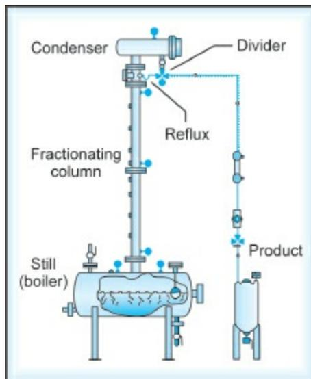
**Fig. 3.18:** Diagrammatic representation of a fractional distillation unit
