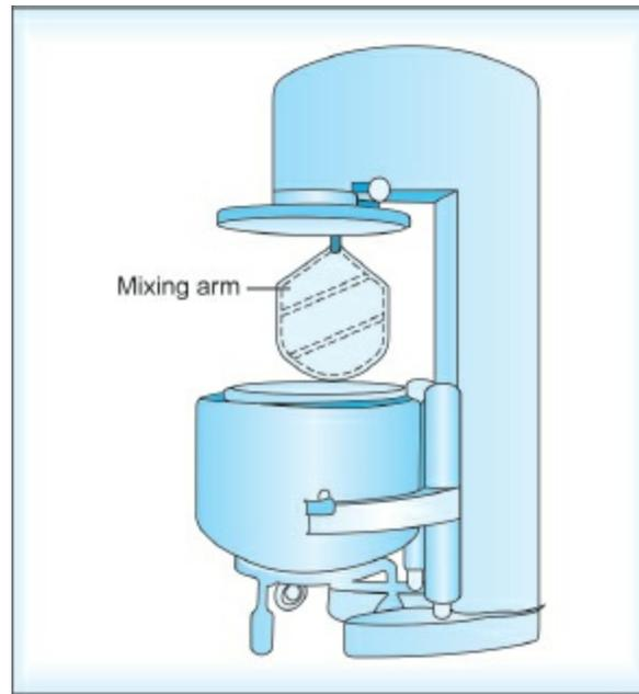
**Fig. 1.13:** Schematic representation of a planetary mixer
