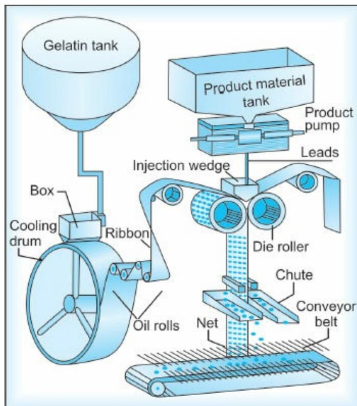
**Fig. 14.24:** Schematic drawing of rotary die process
