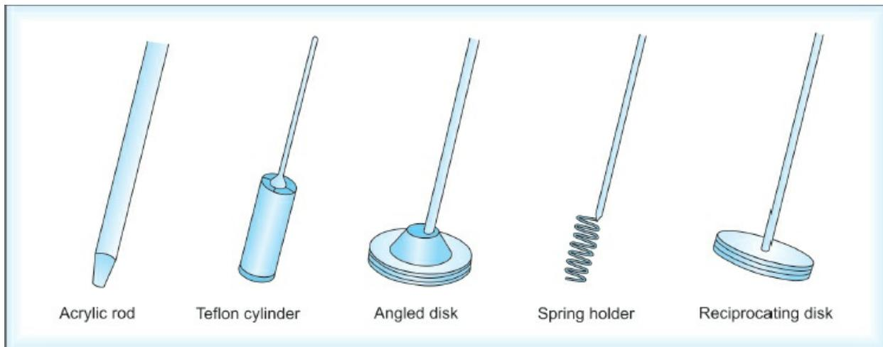
**Fig. 8.11:** Sample holders for dissolution testing of different dosage forms
