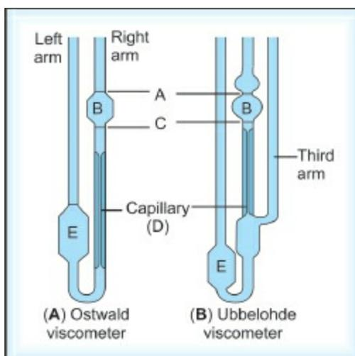
**Figs 6.16A and B:** Capillary or tube viscometers
