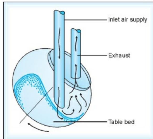
**Fig. 13.23:** Line diagram of standard coating pans
