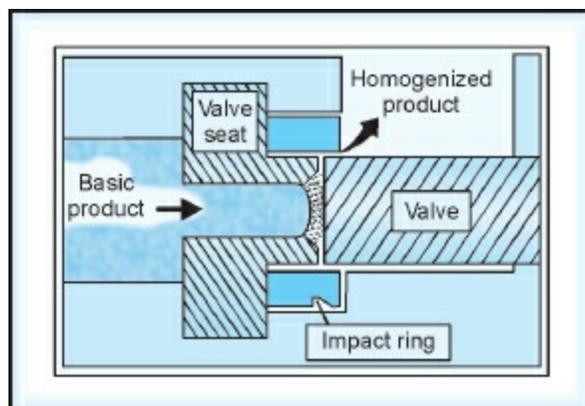
**Fig. 2.19:** Valve assembly of a high-pressure homogenizer
