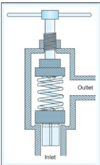
**Fig. 2.16:** Diagrammatic representation of a simple homogenizer
