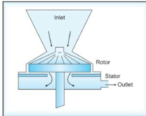
**Fig. 1.16:** Schematic representation of a colloid mill
