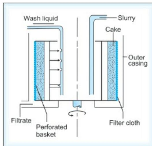
**Fig. 5.14:** Perforated basket type batch centrifugal filter
