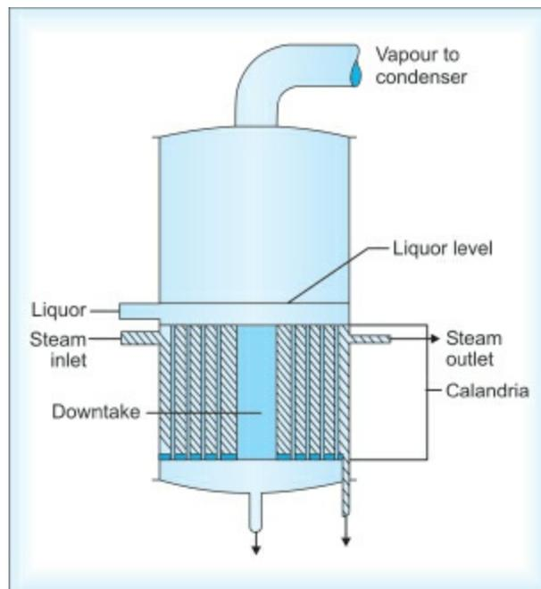
**Fig. 3.5:** Diagrammatic representation of a basket type evaporator
