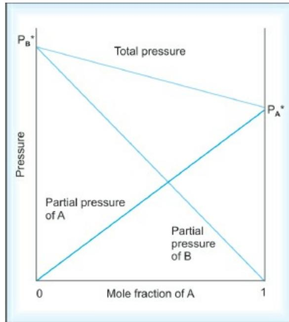
**Fig. 3.12:** Vapor composition diagram for ideal mixtures
