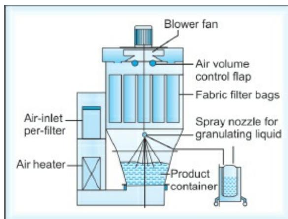
**Fig. 4.13:** Fluidized-bed granulator-dryer
