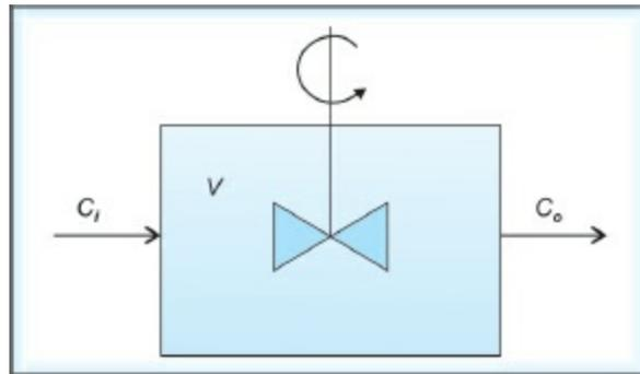
**Fig. 1.8:** Diagrammatic representation of a perfectly mixed tank in a flow stream with a flow rate,  $dv/dt$ .  $C_i$  and  $C_o$  represent the concentrations entering and leaving the tank at any given instant, respectively
