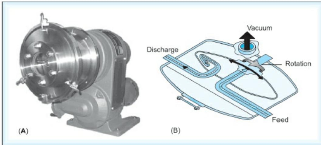
**Figs 26.18A and B:** (A) The Versator consists of a vacuum chamber and a high-speed revolving disc; (B) During operation, material is spread into a thin film by the centrifugal force of the disc, and deaeration is achieved under vacuum (*Courtesy of the Cornell Machine Co*)
