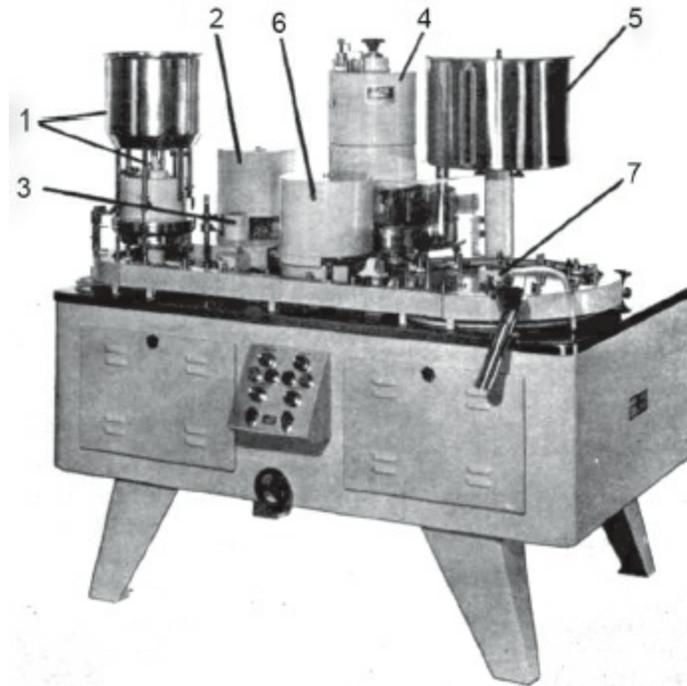
**Fig. 14.10:** MG2 model G36 capsule filling machine, 1. Empty capsule hopper and rectifier, 2. Cap holder removal station, 3. Cleaning station, 4. Powder dosing head, 5. Bulk powder hopper, 6. Cap holder replacing station, 7. Capsule closing and ejection station (*Courtesy of mG2 macchine automatiche, Bologna, Italy*)
