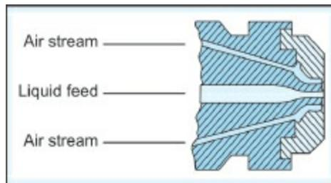
**Fig. 13.33:** Simplified diagram of a low-pressure, air-atomized nozzle
