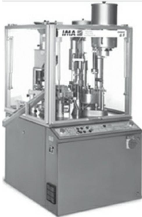
**Fig. 14.14:** Zanasi model 6E capsule filling machine (*Courtesy of Zanasi, SpA, Bologna, Italy*)
