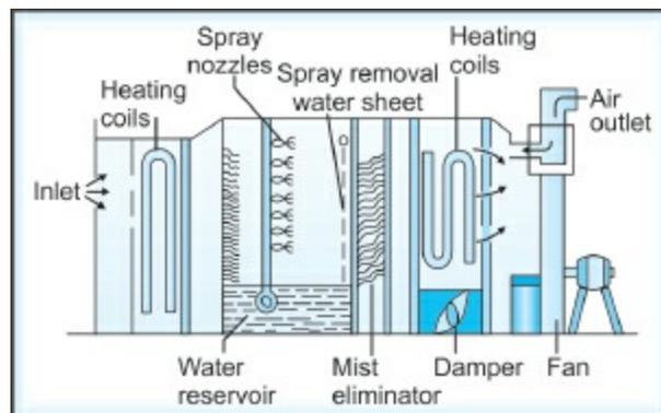
**Fig. 7.9:** Air conditioning unit and control system
