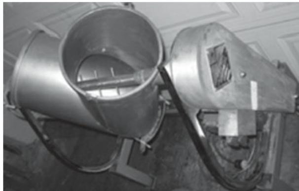
**Fig. 26.7:** Twin shell blender. Material splits and refolds as the blender rotates, producing uniform blends. Various intensifier bars can handle specific applications
