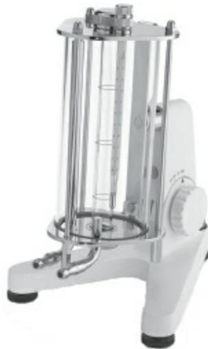
**Fig. 6.19:** Hoeppler falling sphere viscometer
