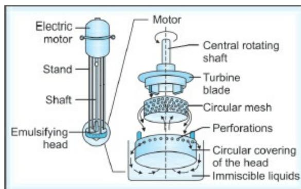
**Fig. 2.17:** Diagrammatic representation of a silverson homogenizer
