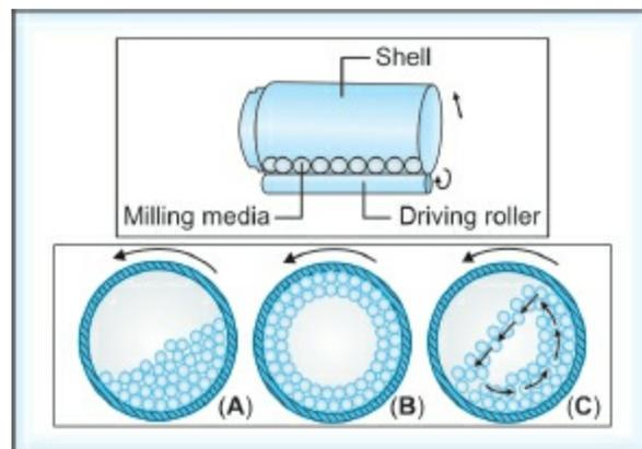
**Figs 2.12A to C:** Diagrammatic representation of ball mill and its operation:
