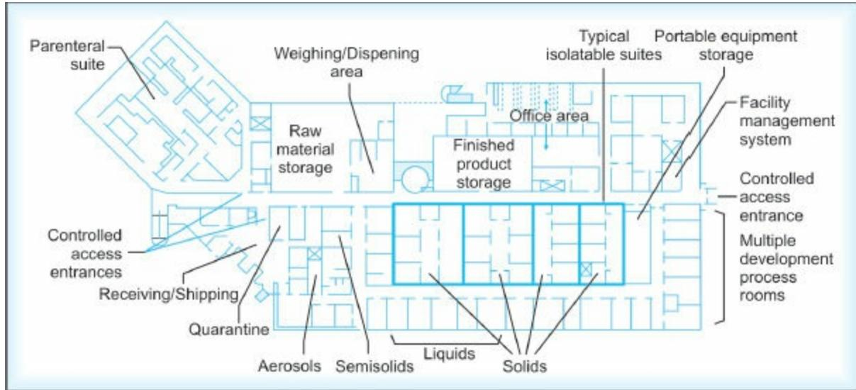
**Fig. 26.2:** A pilot plant layout design
