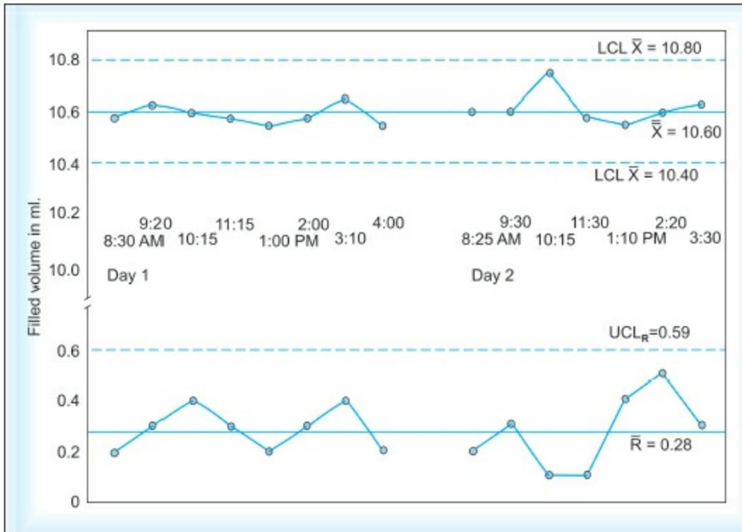
**Fig. 29.6:** Control chart for automatic filling of a parenteral solution in vials. The upper curves are  $\bar{x}$  (mean) charts and the lower curves are R (range) charts.
