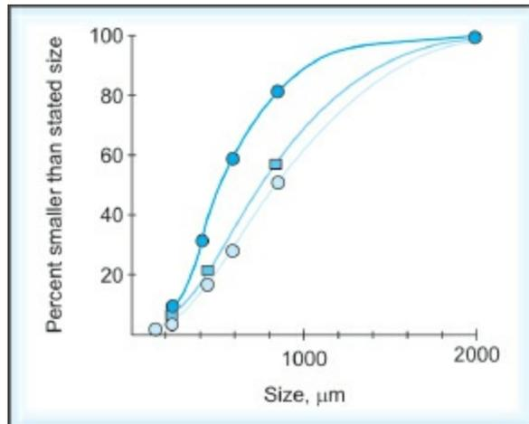
**Fig. 2.8:** Influence of speed on the size-frequency distribution of boric acid flakes milled by a hammer mill operating with impact edge forward and fitted with a round hole No. 4 screen (hole diameter: 6.35 mm). Key:  $\blacksquare$ , 1,000 rpm;  $\circ$ , 2,450 rpm; and  $\bullet$ , 4,600 rpm
