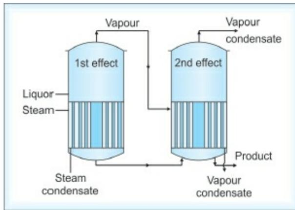
**Fig. 3.6:** Diagrammatic representation of a multiple effect evaporator
