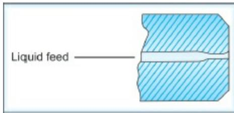
**Fig. 13.32:** Simplified diagram of a high-pressure, airless nozzle
