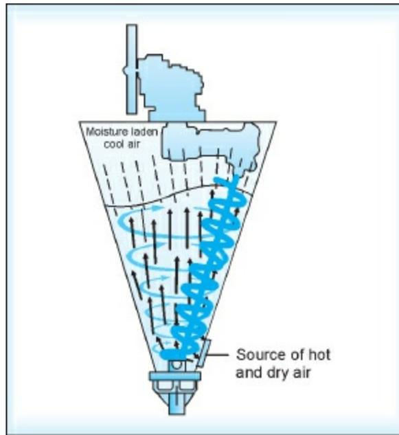
**Fig. 1.20:** Schematic representation of the Nauta mixer
