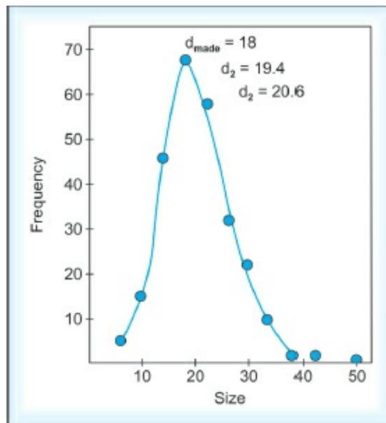
**Fig. 2.23:** Size-frequency distribution of 261 particles measured by microscopy
