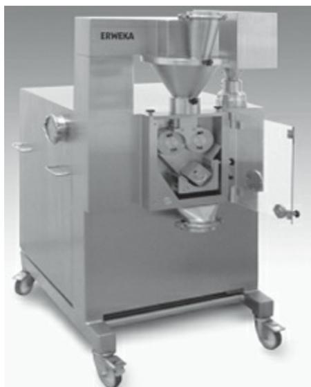
**Fig. 26.5:** Roller compactor for dry compaction operation {*Courtesy of ERWEKA*}
