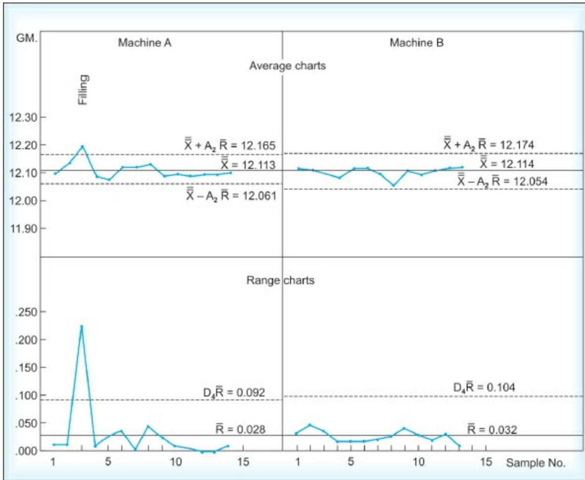
**Fig. 29.8:** Control chart containing the X and R charts on performance of two filling machines after process investigation and improvement. Note that the control limits were narrowed on  $\bar{X}$  and R charts as compared to that of [Figure 29.7](#)
