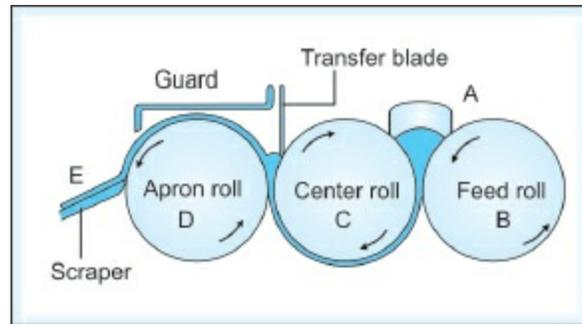
**Fig. 1.15:** Cross section of a three-roller mill
