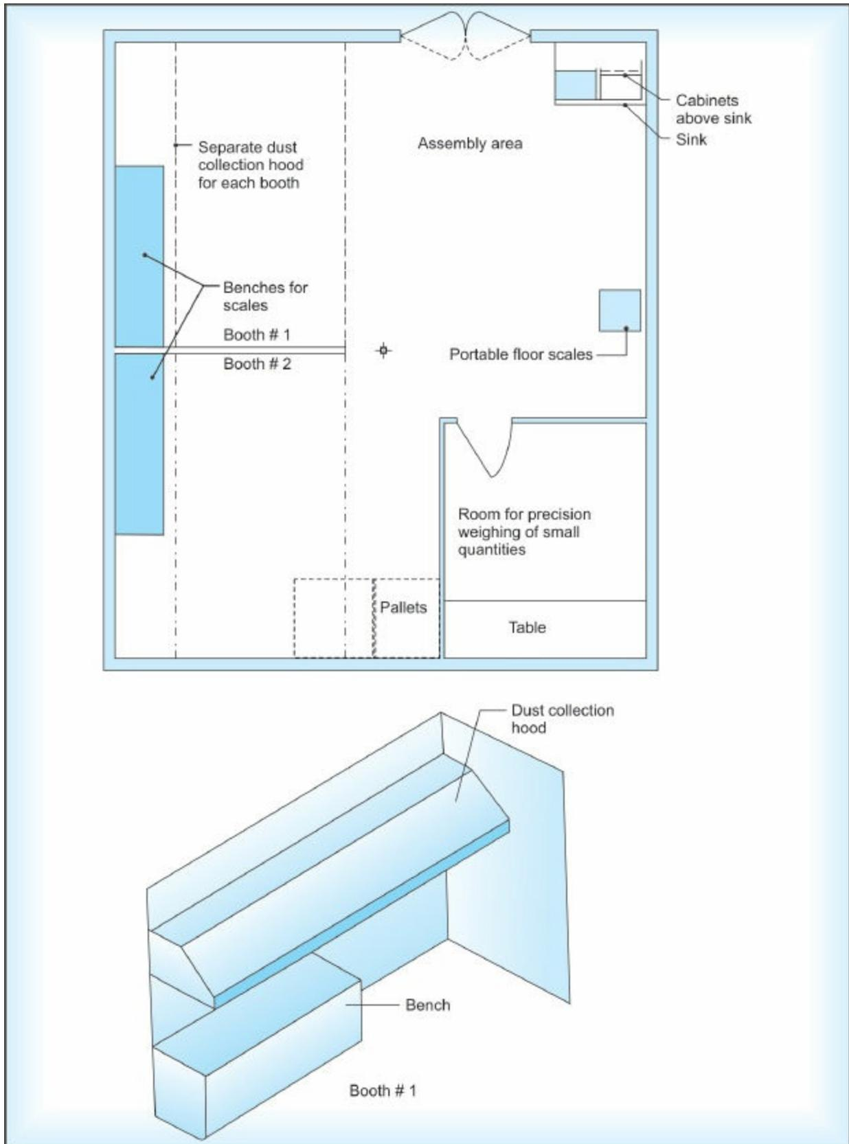
**Fig. 26.4:** Top, two weighing booths together with enclosed room for weighing steroids and the like. Bottom, workbench and hood, which should be connected to dust collector
