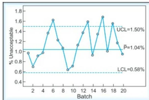
**Fig. 29.10:** Control chart (p chart) for percentage of broken tablets in plastic
