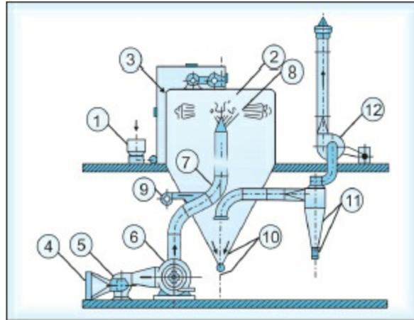
**Fig. 4.15:** Spray dryer: 1. feed tank; 2. centrifugal atomizer; 3. drying chamber; 4. inlet air filter; 5. air supply fan; 6. air heater; 7. triple inlet duct; 8. adjustable air disperser; 9. cooling air fan; 10. chamber product collection; 11. cyclone product collection; 12. exhaust fan
