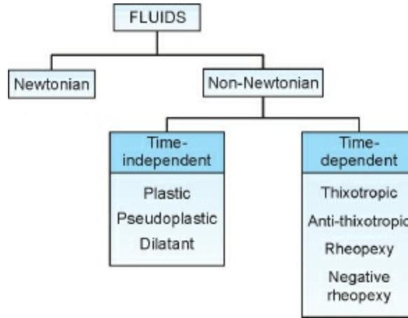
**Fig. 6.2:** Classification of fluids based on rheological behaviour
