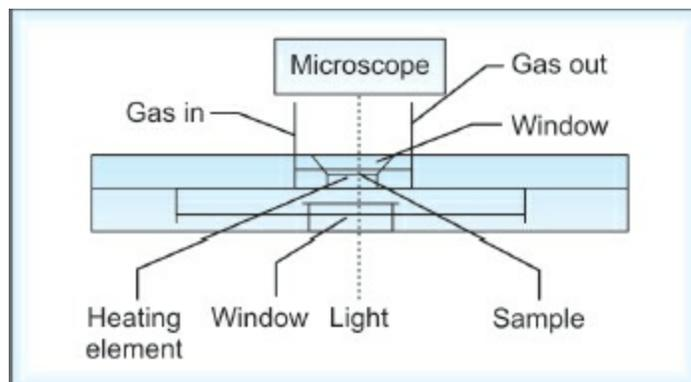
**Fig. 9.17:** Schematic diagram of a hot stage microscopy
