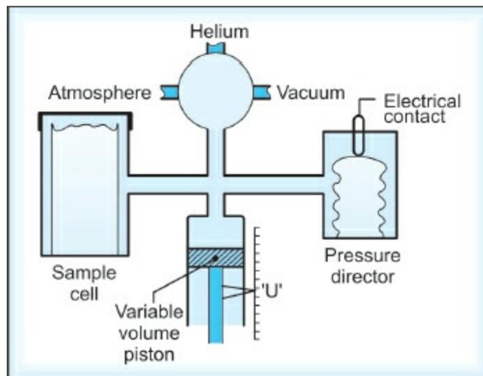
**Fig. 9.24:** Diagram of a helium pycnometer for determining the true volume of powders. The variable volume piston positions ( $U_1$ ,  $U_2$ , and  $U_3$ ) are read off from the scale and are used in equation (6) (see text)
