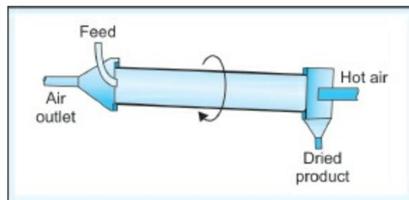
**Fig. 4.11:** Rotary dryer
