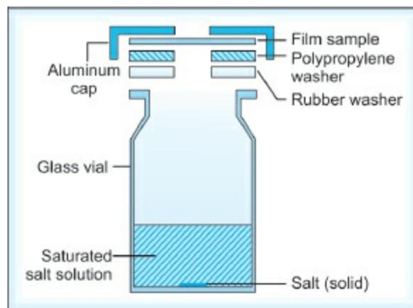
**Fig. 13.37:** Schematic of a water vapor transmission cell
