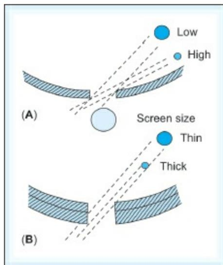
**Figs 2.9A and B:** In a hammer mill: (A) Particle size is influenced by speed, (B) Thickness of screen
