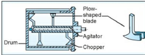
**Fig. 1.21:** Diagrammatic representation of the Lödige mixer
