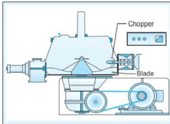
**Fig. 1.22:** Diagrammatic representation of the Diosna mixer
