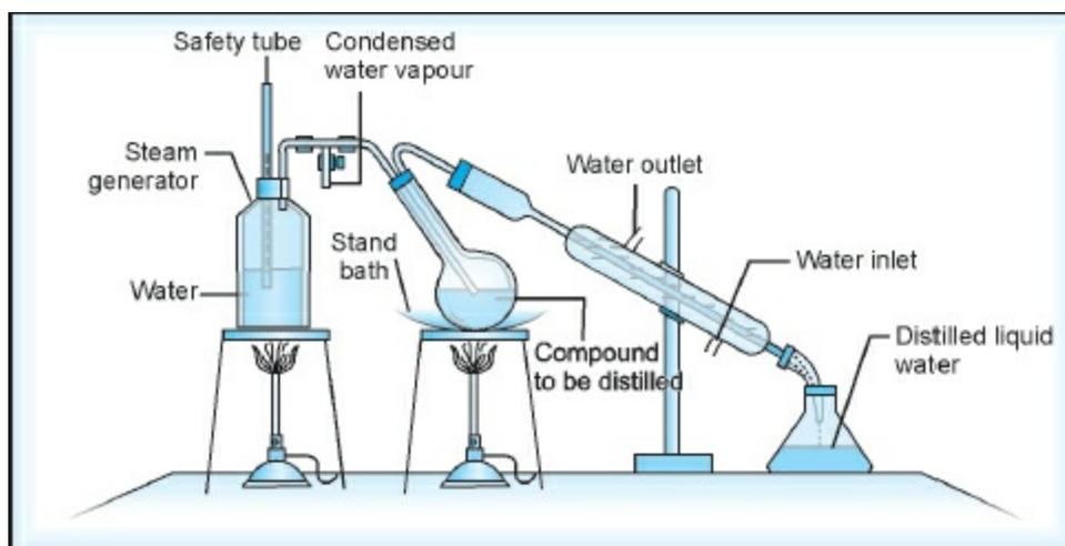
**Fig. 3.22:** Diagrammatic representation of a steam distillation unit
