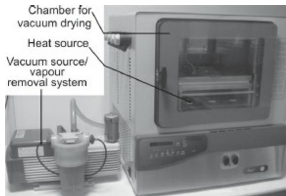
**Fig. 4.7:** Schematic representation of a Freeze dryer
