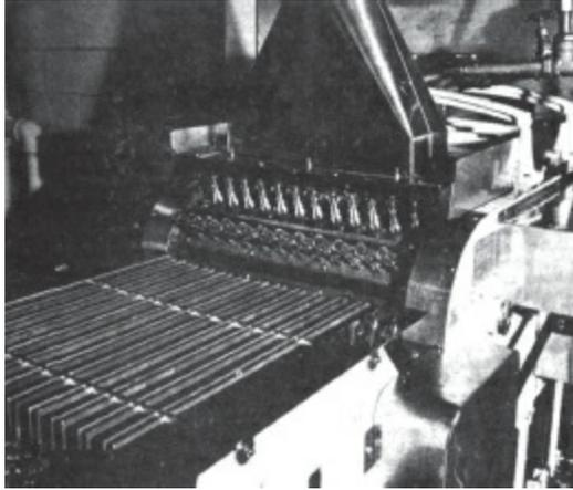
**Fig. 23.8:** Conveyor rinser delivering clean vials to an adjoining clean room
