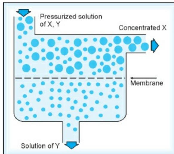
**Fig. 5.19:** Schematic diagram of membrane ultrafiltration process
