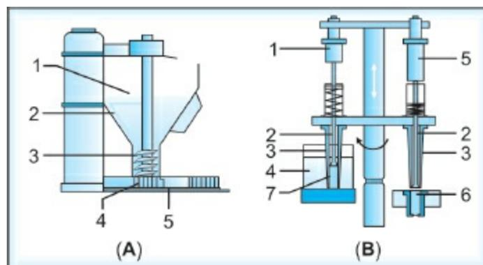
**Figs 14.4A and B:** Feeding mechanisms of the capsule filling machine: (A) Auger feeding unit (1) powder hopper, (2) stirrer, (3) auger, (4) body holder, (5) turn table; (B) Dosator feeding unit (1) compression force, (2) piston, (3) dosing tube, (4) powder hopper, (5) plug ejection plate, (6) capsule body, (7) powder plug
