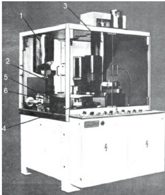
**Fig. 14.8:** H and K Model 602 capsule filling machine, 1. Empty capsule storage hopper, 2. Rectifier, 3. Bulk powder storage hopper, 4. Capsule body transport segment, 5. Closing station and 6. Filled capsules ejection station
