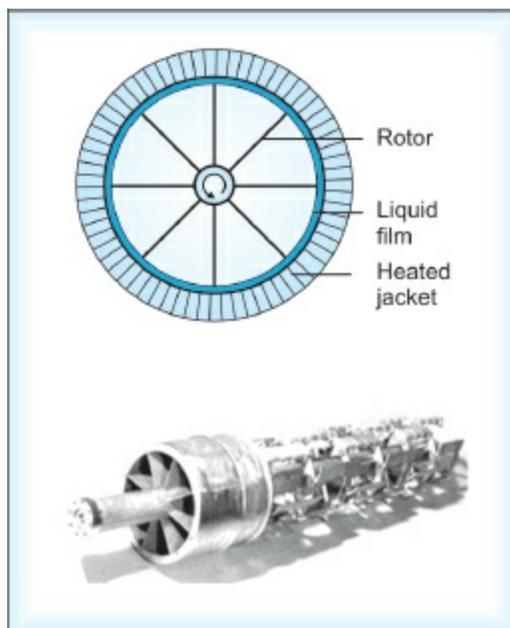
**Fig. 3.9:** Cross section of SAMBAY<sup>®</sup> wiper film evaporator and SAMBAY<sup>®</sup> rotor
