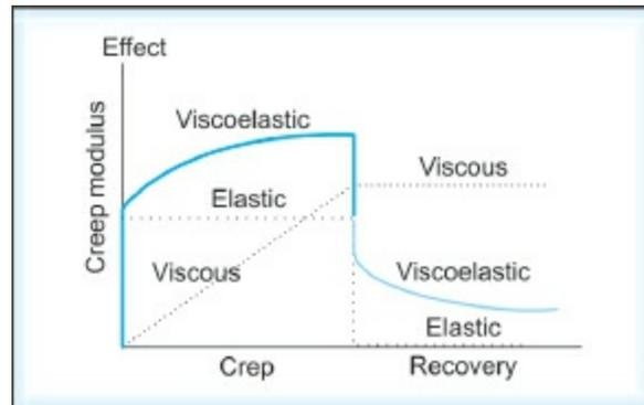
**Fig. 6.31:** Creep curve for a viscoelastic material
