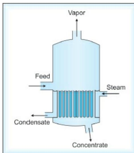
**Fig. 3.4:** Diagrammatic representation of a standard evaporator with
