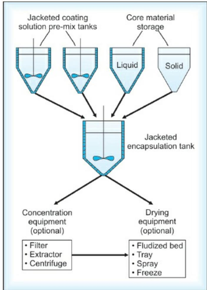
**Fig. 15.15:** Flow diagram of a typical phase-separation/coacervation process
