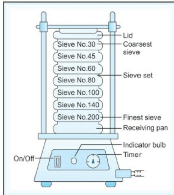
**Fig. 2.26:** Arrangements of sieves in sifter
