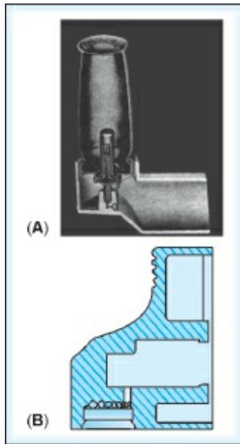
**Figs 21.4A and B:** Actuators for pharmaceutical aerosols: (A) Inhalation spray type (*Courtesy of Riker Laboratories*); (B) Mechanical breakup type (*Courtesy of Risdon Manufacturing Co., Naugatuck, CT*)
