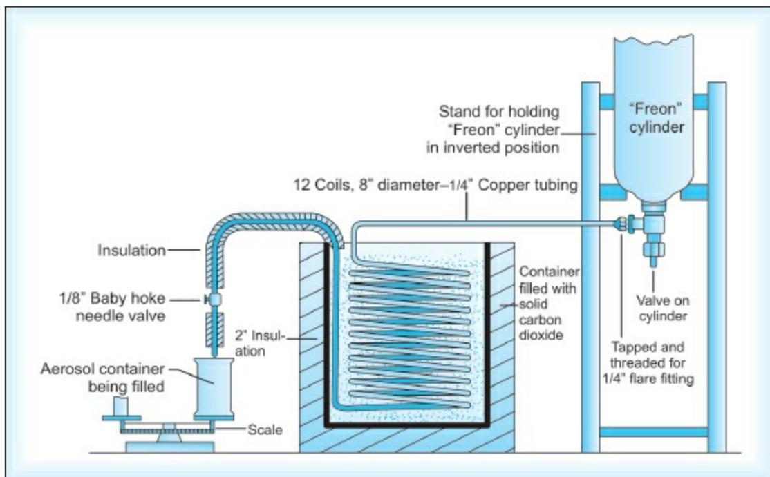
**Fig. 21.11:** Apparatus for cold filling process (Courtesy of EI. duPont de Nemours and Co., Inc., Wilmington, DE)
