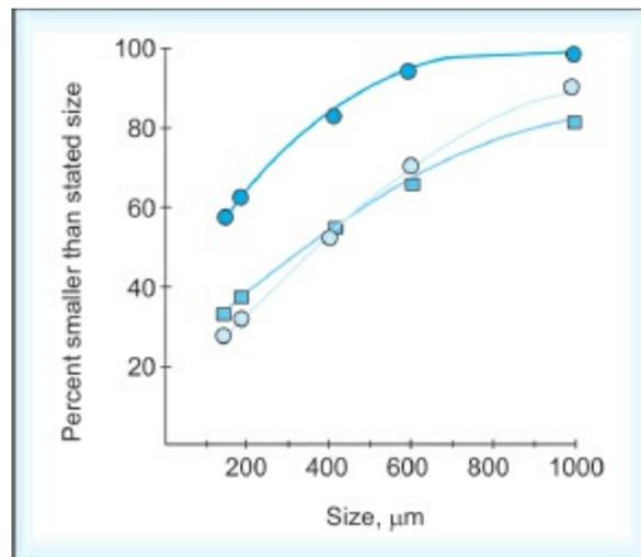
**Fig. 2.10:** Influence of screen size on the size-frequency distribution of a *Terra alba* granulation milled with a hammer mill operating at 2450 rpm, and a comparison with the granulation milled by a vertical hammer mill fitted with a no. 10 screen. Key: ○, hammer mill, 0.84 mm; ● hammer mill, 1.65 mm; and ■, vertical hammer mill
