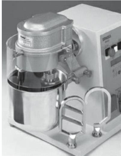
**Fig. 26.6:** Planetary mixer (Courtesy of ERWEKA)
