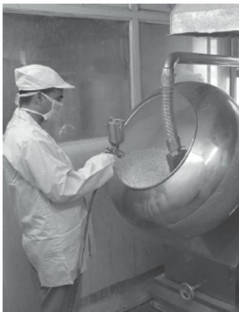
**Fig. 13.34:** Coating of tablets in a pharmaceutical setup (*Courtesy of Unicare*)
