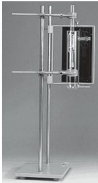
**Fig. 20.5:** Suppository melting point apparatus (Courtesy by permission from ERWEKA<sup>®</sup>)
