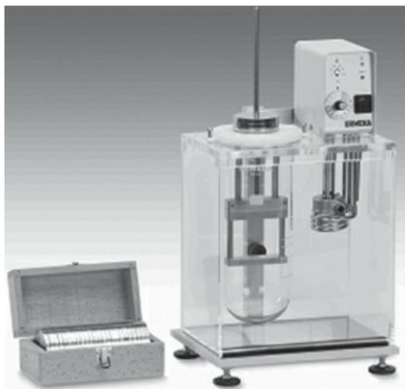
**Fig. 20.7:** Breaking test apparatus (*Courtesy by permission from ERWEKA<sup>®</sup>*)
