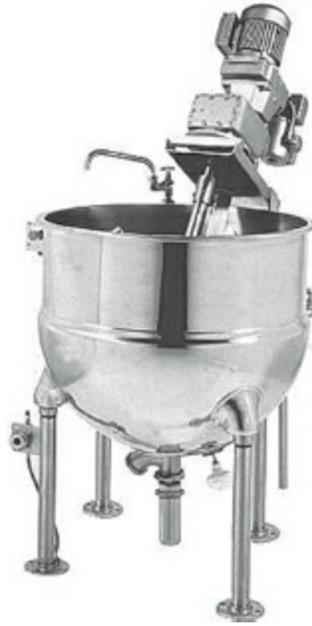
**Fig. 19.8:** Stainless steel jacketed mixing kettle equipped with a slow-speed, anchor-type sweep blade agitator which takes the material from the side wall and swirls it around this secondary bar type mixer
