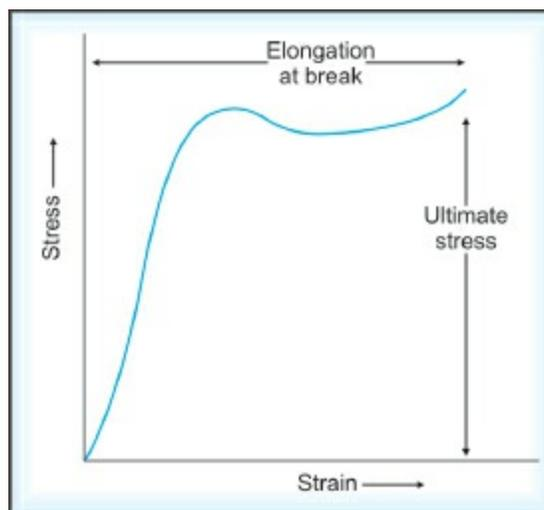
**Fig. 13.38:** Example of a stress-strain curve obtained in the tensile testing of
