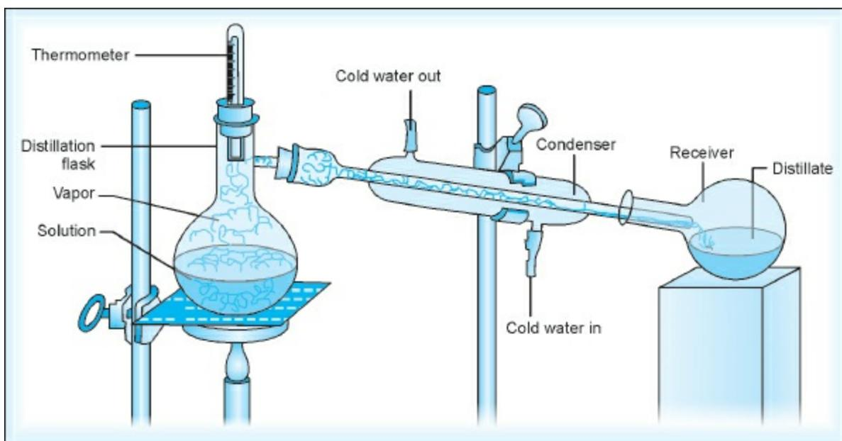
**Fig. 3.16:** Set up of a simple distillation unit
