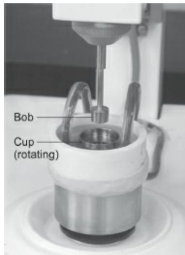
**Fig. 6.20:** Couette type cup and bob viscometer
