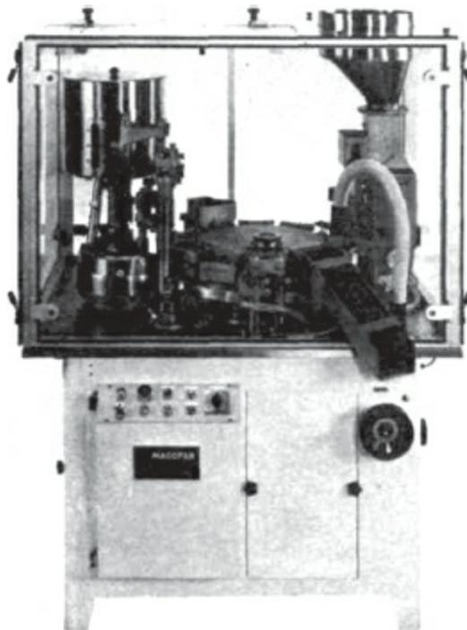
**Fig. 14.9:** Macofar model MT-12 capsule filling machine (*Courtesy of Macofar, Bologna, Italy*)
