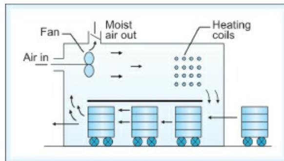
**Fig. 4.8:** Tunnel dryer
