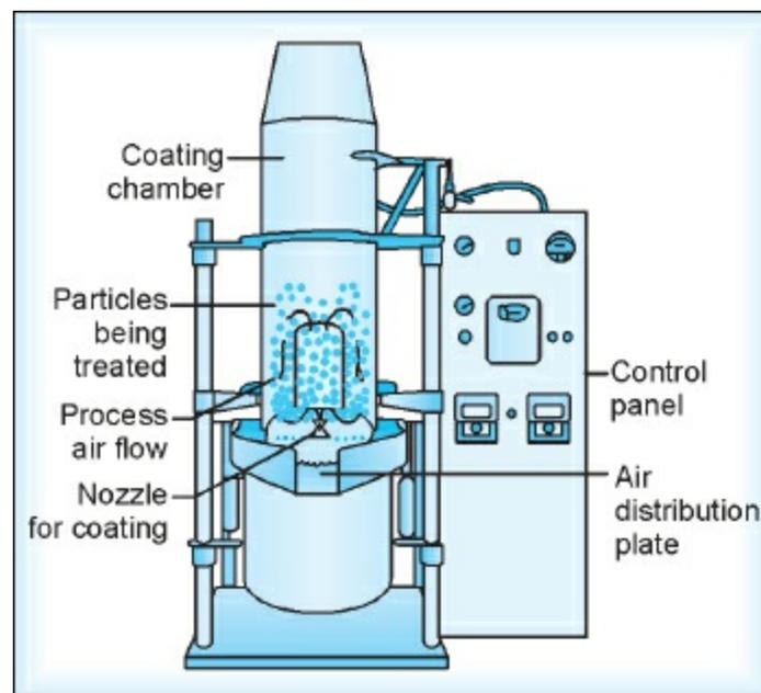
**Fig. 15.8:** Schematic drawings of Wurster air suspension apparatus
