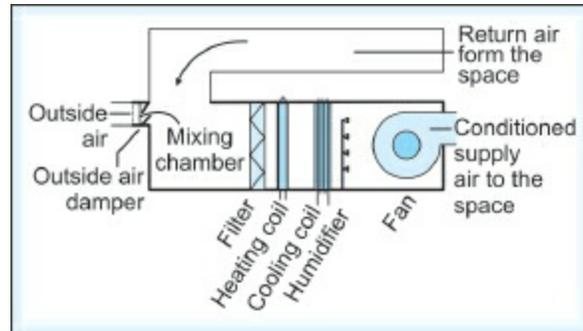
**Fig. 7.8:** Schematic representation of air conditioning cycle
