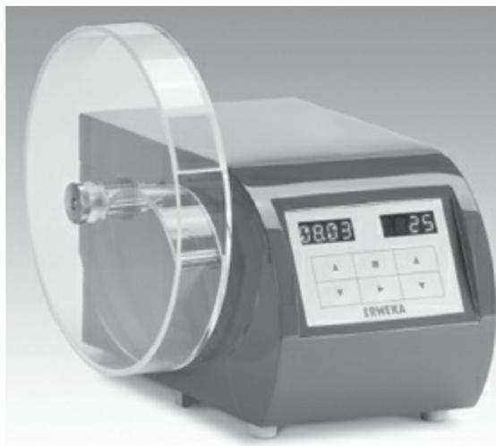
**Fig. 13.13:** The friability apparatus (Courtesy of ERWEKA)
