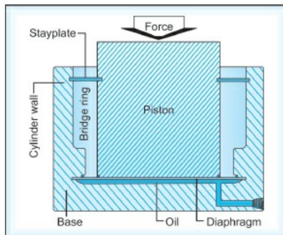
**Fig. 19.6:** Schematic diagram of a cross-section of a hydraulic load cell
