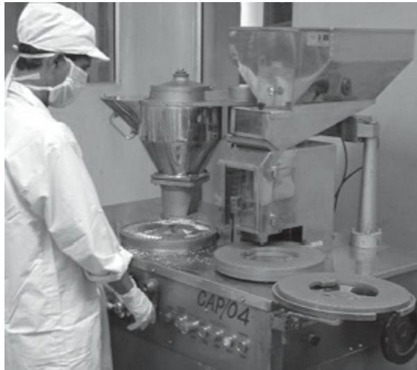
**Fig. 14.3:** Filling of hard two-piece capsules (*Courtesy of Unichem*)
