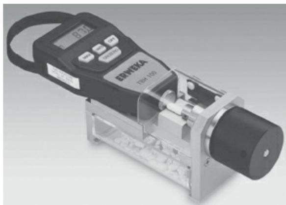
**Fig. 13.12:** The Erweka tablet hardness tester (*Courtesy of ERWEKA*)
