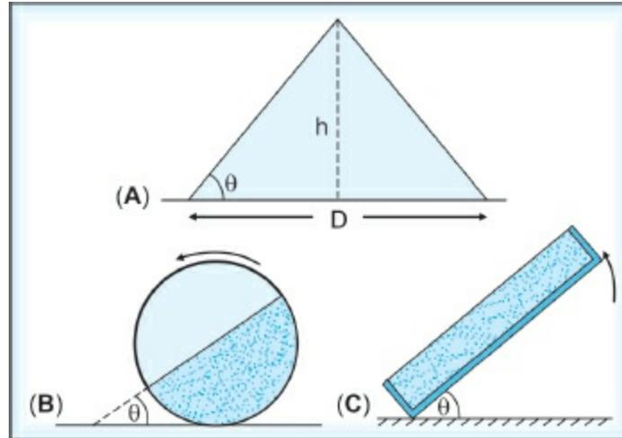
**Fig. 9.26:** Measurement of dynamic angles of repose,  $\theta$ , as defined from the dimensions of a conical bed of the powder (A), where  $\tan\theta = \frac{2h}{D}$  (twice the powder bed height (h)/powder bed diameter (D)). (B and C) represent the rotating cylinder and tilted box methods of measurement, respectively
