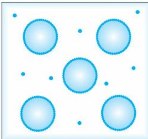
Step 2: Deposition of liquid coating material
