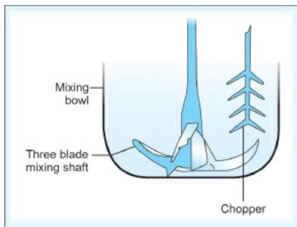
**Fig. 1.23:** Diagrammatic representation of the Gral mixer-granulator
