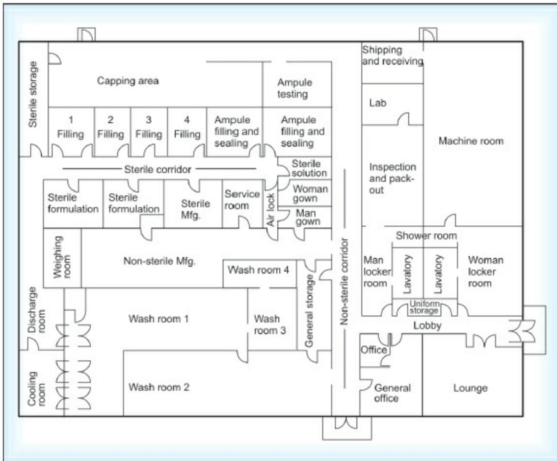
**Fig. 23.5:** Floor plans for industrial sterile products production area
