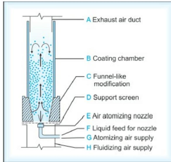
**Fig. 13.31:** Line diagram of a fluidized bed coater
