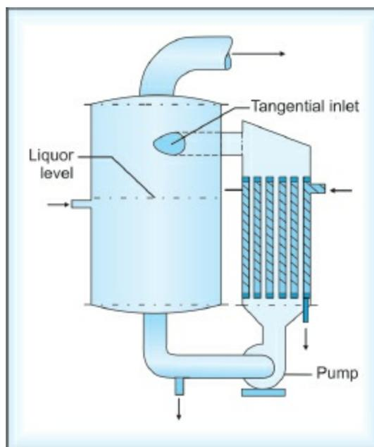
**Fig. 3.8:** Diagrammatic representation of a forced circulation evaporator
