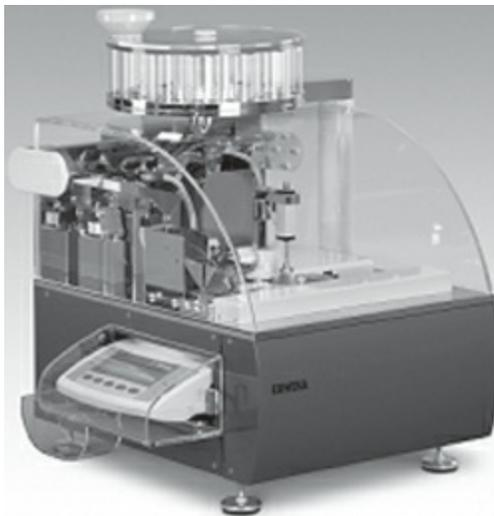
**Fig. 26.16:** Multicheck apparatus for tablet testing (*Courtesy of ERWEKA*)
